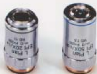
LWD (LONG WORKING DISTANCE) PLAN EPI OBJECTIVES
